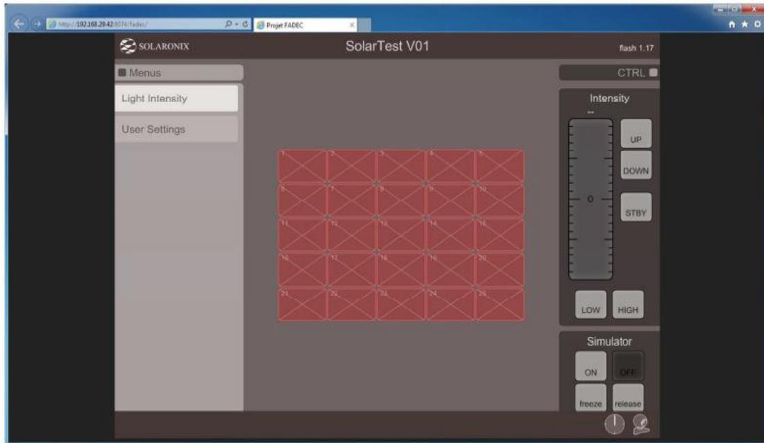
Example of lamps array remote control
