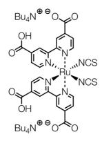
For industry or researchers who manufacture or study Dye Solar Cells, Ruthenizer 535-bisTBA is a high performance ruthenium dye which very efficiently sensitizes wide bandgap semi-conductors like titanium dioxide.
