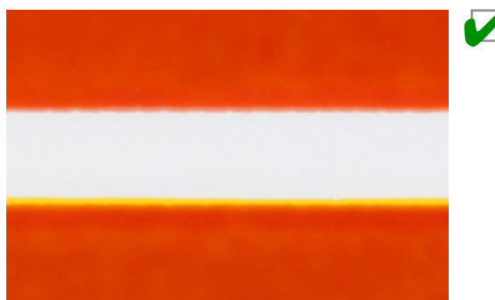
Example of a good sealing, showing the absence of noticeable defects in the gasket.
