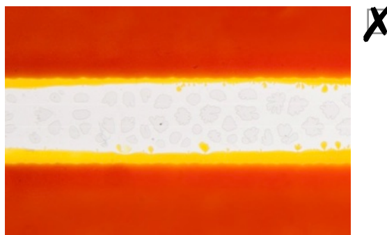
The bubbles present in the sealing gasket will eventually cause leakage.
