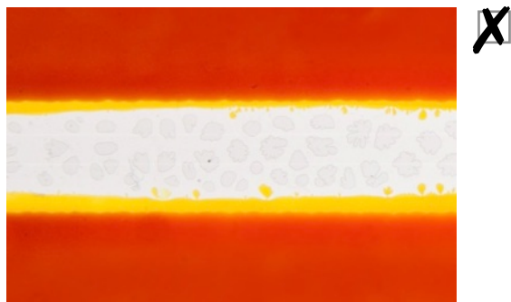
The bubbles present in the sealing gasket will eventually cause leakage.
